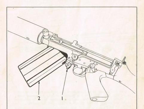
Press the magazine catch 1 and push the magazine 2 forward to remove it.
