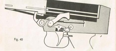
When the change lever is put to R the flat surface is immediately above the rear arm of the trigger. The hammer is held by the nose of the sear engaging in the bent. The rifle is ready to fire.
