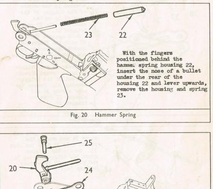
Lift the free end of the locking plate 24 upwards as far as possible, push out the hammer axis pin 25 and remove the hammer.
