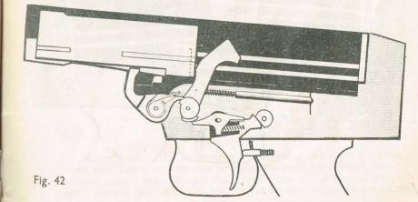
During the backward movement the rear bottom surface of the breech block slide rotates the hammer to the rear and downwards.
