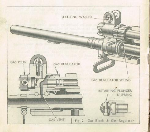
If the letter A on the plug is turned uppermost, it indicates that the rifle is set for ball ammunition firing, in this position, the gas port in the plug is directly in Line with the gas vent in the barrel.
