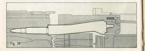
The slide continues its forward movement and immediately before reaching its limit of travel a projection on the rear bottom surface of the slide comes into contact with the upper arm of the safety sear, and trips it forward releasing the nose of the safety sear from the upper bent of the hammer. The hammer rotates forward until the lower bent is engaged
