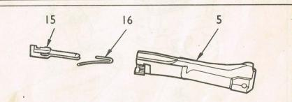
Put the nose of a bullet under the claw of the extractor 15 and push outwards as far as possible, lever up the extractor 15 clear of the block 5. Push on the long arm of the extractor spring 16 to disengage it from the extractor 15.
