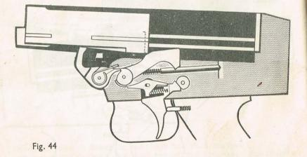
As the breech block moves forward the hammer follows until the upper bent contacts the safety sear.
