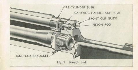
A bush is fitted over the rear end of the gas cylinder. Grooves on the outer surface of the bush allow the use of a tightening tool.
