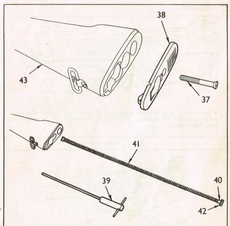
Unscrew the butt plate screw 37 and remove the butt plate 38. Using the special tool provided 39, remove the return spring screw 40 and withdraw the return spring 41 and washer 42.
