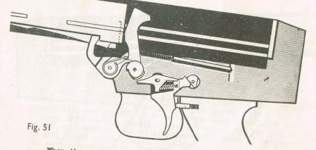
When the safety sear is tripped the hammer is released and goes forward to strike the firing pin. The rifle will continue to fire at the automatic rate until the trigger is released or the magazine is emptied.
